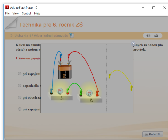
Pic.4: Correct connection of bulbs in series, solution of electronic task nr.4 (source: own suggestion)
