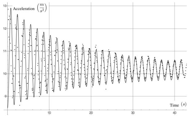
Figure 2: Plot of the measured smartphone acceleration (orthogonal to the smartphone screen) and the corresponding approximate solution of the differential equation that models the pendulum.
