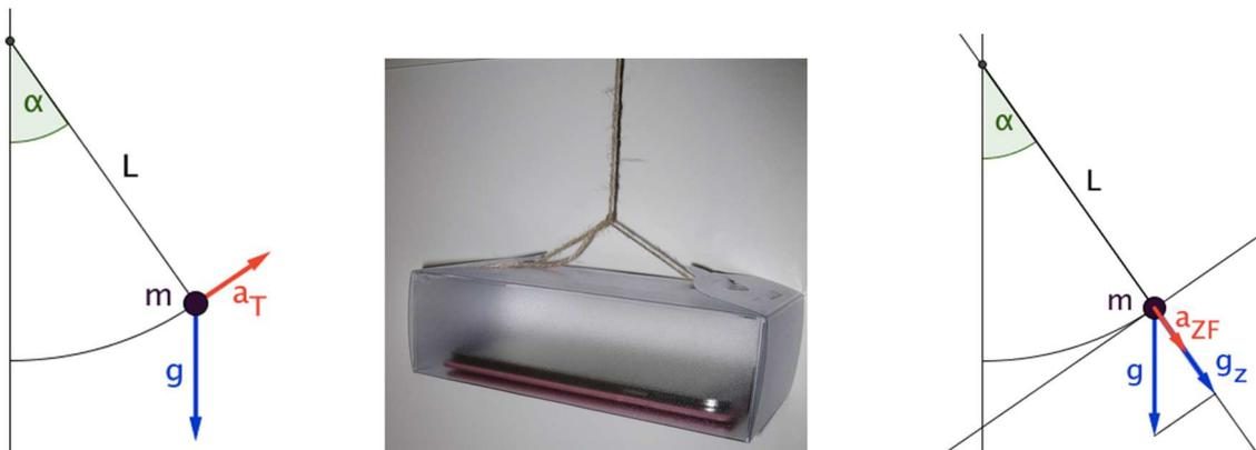
Figure 1: Left and right: Schematic drawings of a pendulum showing the relevant acceleration components. Middle: Smartphone in a plastic box, used as the bob of a pendulum.
