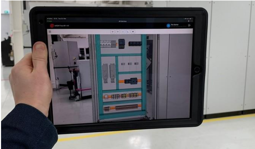
Fig. 3. Virtual switchboard with the real switchboard in the background (Source: https://www.vseoprumsylu.cz/digitalizace/virtualni-rozsirena-realita/digitalni-rozvadec-primo-na-stole-eplan-eview-free-nyni-s-ar-funkcemi.html )
